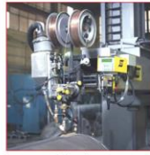
Twin-wire Single Arc SAW
