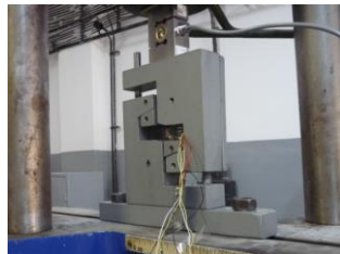
Figure 1: Shearing tests with Iosipescu Fixture System
