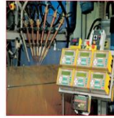
Multiple wires SAW: (six wires - same welding pool)
